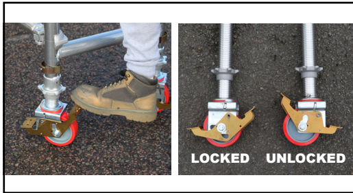
3. Lock Brakes and allow 3" thread from bottom of castor for levelling
